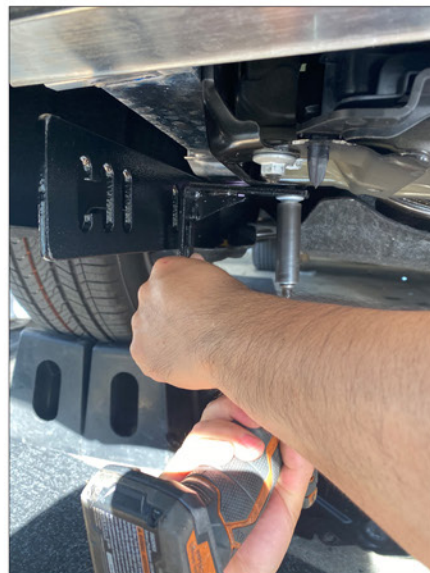
4.Secure with an air gun.
