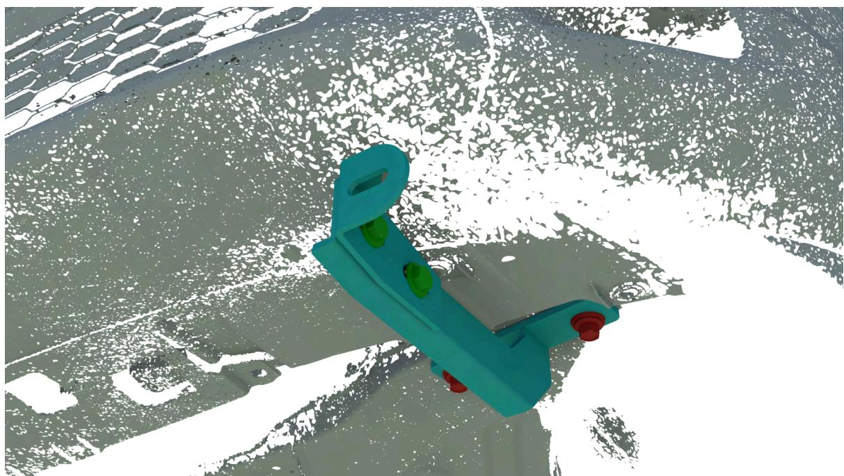
Step4: Bumper Guard (A) installation with screws (D/F/G).
