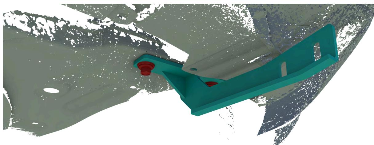
Step3:Mount Adapter Bracket (C) onto the Bracket (B), use Screws (D/E/F/G) to fix them.
