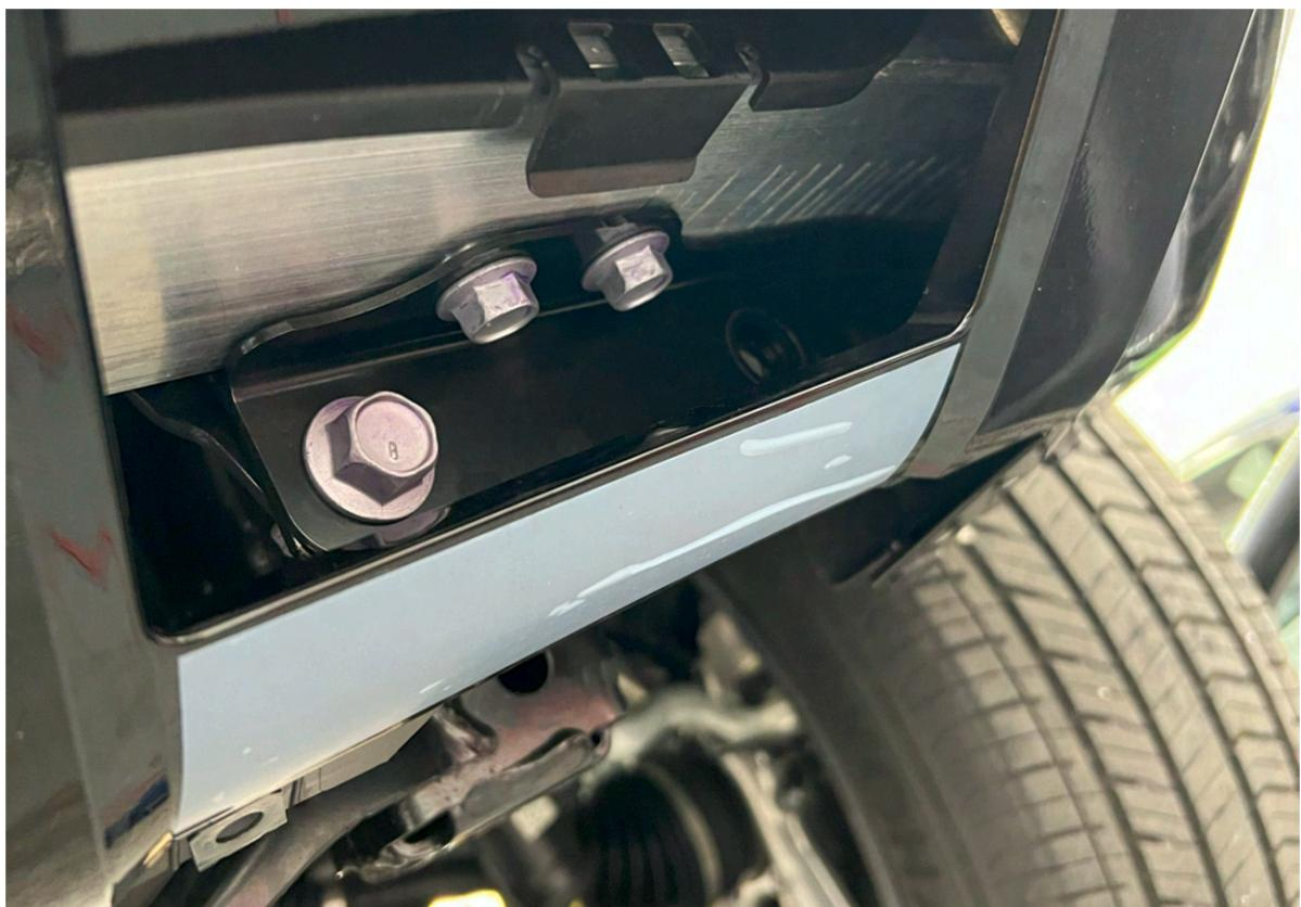
Step5: Mount Support Bracket (C) onto the car, use the original car bolt to fix it.
