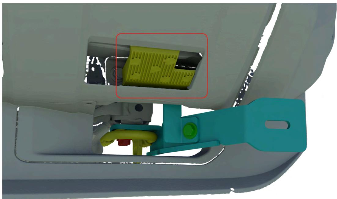
Step8: Bumper Guard (A) installation with screws (D/F/G).
