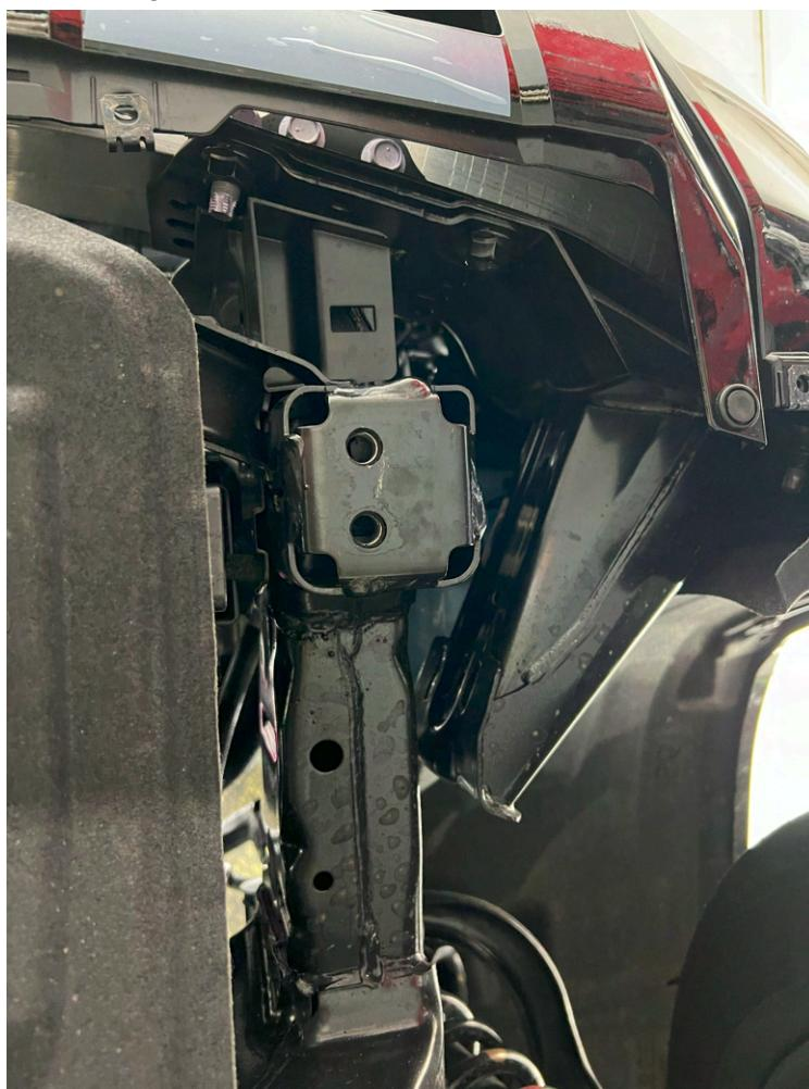
Step2: Mount the Bracket (B) onto the car, and put the trailer hook and Bracket (B) together, use original car bolts to fix it.
