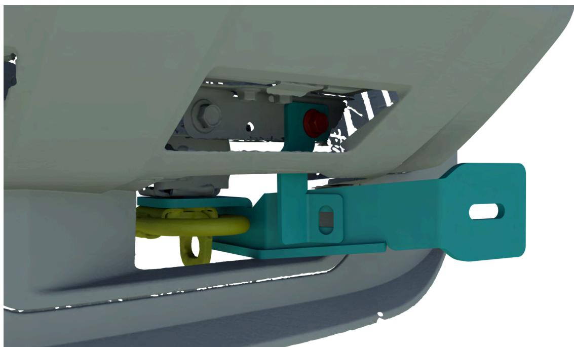
Step6: Use Screws (D/E/F/G) to fix Bracket (B) and Support Bracket (C).
