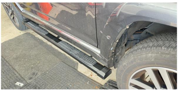
Mounting the **FRONT** bracket to the car shown in the picture.
