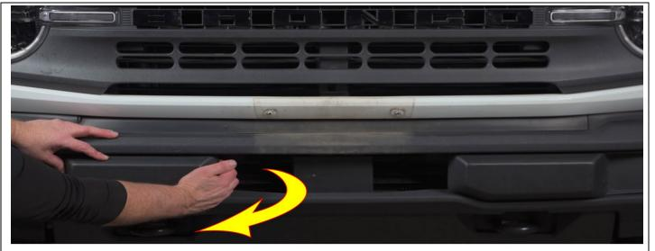
Pull the plastic cover off and lock the bracket in place with the original three screws. It is recommended to install one side before
