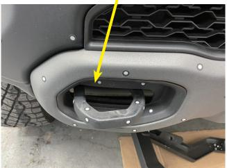
Place the iron tabs on the top and bottom of the trailer hitch and secure with screws
