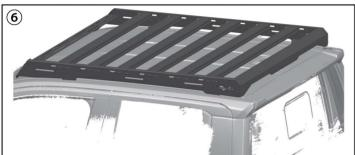
Align the rear side beams with the left and right side beams in the holes, put in the washers, thread in the screws, and secure them with the nut locks.
