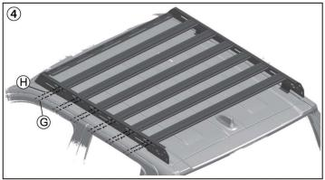
Place the hole bracket on the roof of the car, adjust the position, and tighten it with washers and screws. (Apply sealant to screws)
