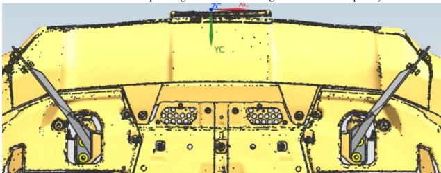
Step4:Install the bar body on the bracket and adjust the mounting position of the bracket according to the position of the bar body.
