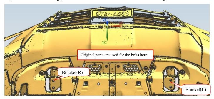
Step 3:Attach the bracket to the corresponding holes but do not tighten the standard parts yet.
