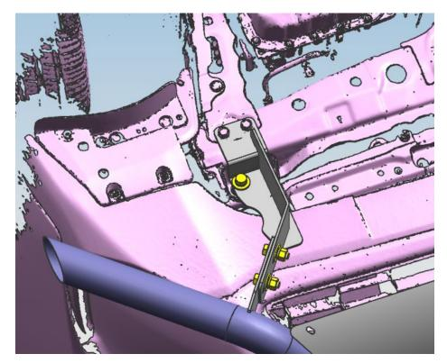
Step 3:Attach the bracket to the corresponding holes but do not tighten the standard parts yet, after that install the bar body on the bracket and adjust the mounting position of the bracket according to the position of the bar body.
