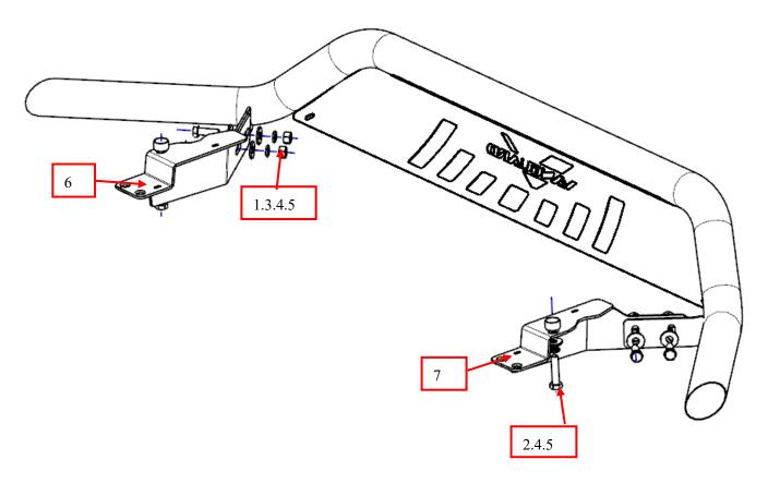
Step 1: Refer to the Part list to check if all the hardware are included. Step 2:Refer to the following pictures to assemble brackets on the main tube (left/right).
