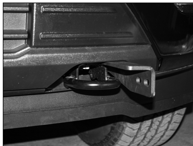
(Fig 6 Driver/left side Frame Bracket installed without tow hook
