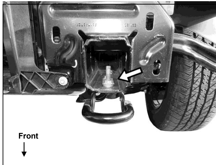
(Fig 2) Temporarily remove tow hooks if equipped
