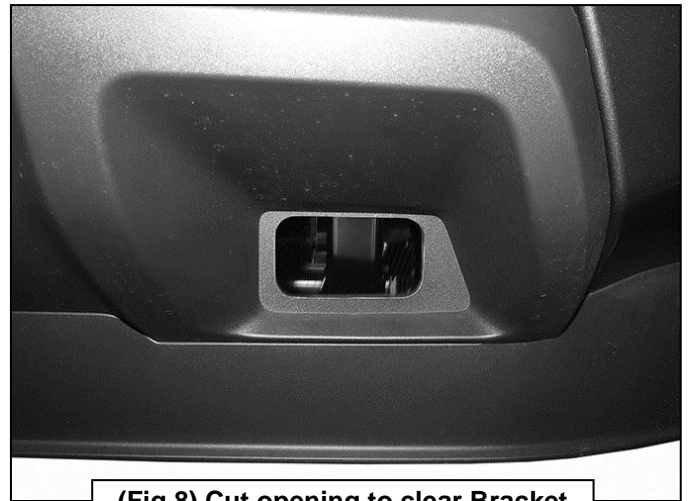
(Fig 8) Cut opening to clear Bracket
