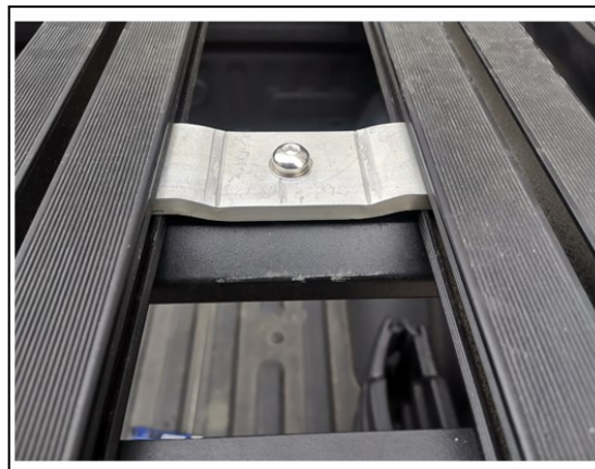
5. Slide the accessories into the base plate, adjust the frame and crossbeam to a proper position, and then lock them with screws
