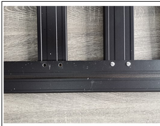
3. Install the bottom plate, match the bottom plate to the hole of the frame, and fix it with screws.
