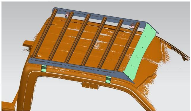
5. Adjust the position of the bracket and tighten all the screws
