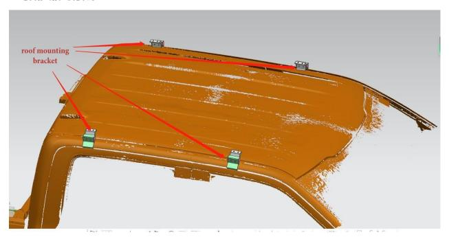
4. Put the assembled luggage frame on the roof bracket and fix it with screws
