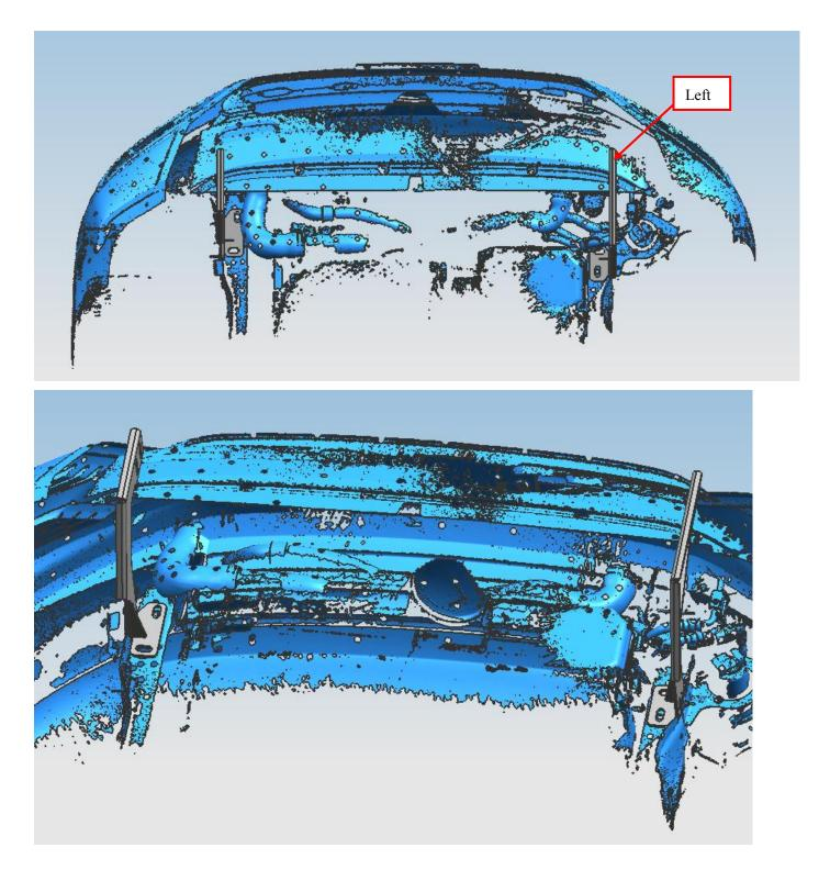
Step 3:Install the bracket on the corresponding hole position, but do not tighten the standard parts yet.Install the bull bar on the bracket and adjust the installation position of the bracket according to the position of the bull bar.
