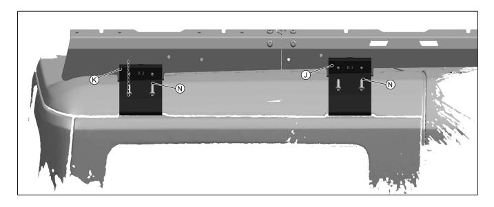
5 Install the spotlight bracket and lock 4 screws.
