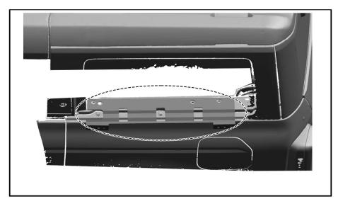
As shown in the figure, install the right iron bracket to fix the right suspension roof ladder. Note: If it is not necessary to install the side roof ladder, skip this step.
