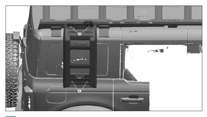
2 Install the plastic cover on the upper side of the roof ladder.
