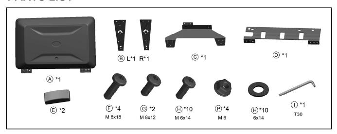
1: To install the storage box, install the roof blade platform and the lower iron bracket. 2:Assemble the upper iron bracket and lock 6 screws.
