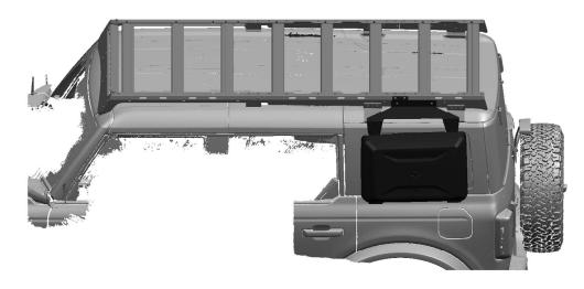
According to the number on the bracket, connect the three sections of bracket as a whole, distinguish left from right, and install the whole bracket on the roof.
