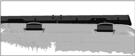
Install the iron clips on both sides, and distinguish the directions.
