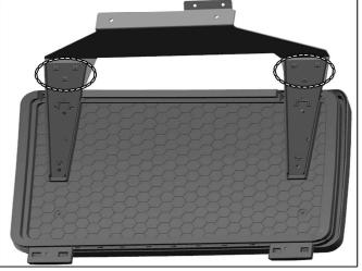
1: As shown in the figure, install the storage box, lock 4 screwson the upper side and 2 screws on the lower side. 2:Install 2 plastic covers under the storage box.
