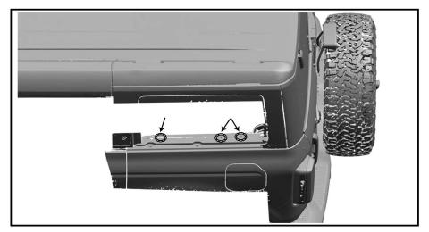
As shown in the figure, install the left iron bracket to fix the left suspension storage box. Note: If it is not necessary to install the side storage box, skip this step.
