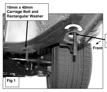
12mm x 90mm Bolt Plate (twist 90-degrees)
