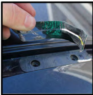
You can either trim around the holes or remove the whole sticker
