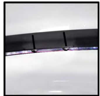
Alternately you can mark at the center of the holes if you wish to make exact holes for the spacers. This technique will be covered second
