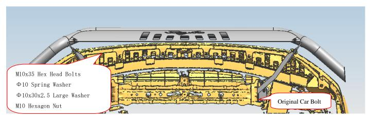
Step 4: Check if all hard ware are installed and then fasten all to complete the installation.
