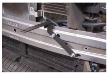
Attach (2) Upper Brackets to the bumper beam. Fasten with (1) 5/16' Flat Washer, Lock Washer, and Hex Nut on each Bolt Plate.
