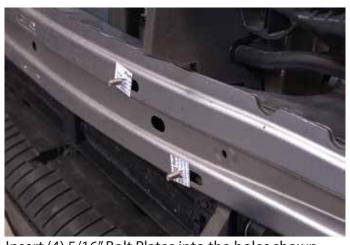
Insert (4) 5/16" Bolt Plates into the holes shown. Slide the Bolt Plates towards the center of the vehicle.
