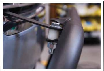
Attach the Light Bar as shown with (1) 3/8" x 1.75" Hex Bolt, (1) Flat Washer, (1) 3/4" Nylon Spacer, (1) Flat Washer, (1) Lock Washer, and (1) Hex Nut per side.
