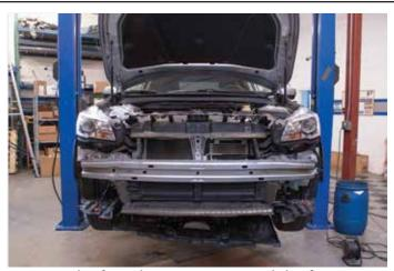
Remove the front bumper cover and the foam piece in front of the bumper beam.
