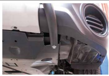
Cut the splash guard by following the outer crease until the bar clears.
