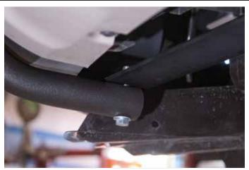
Attach the Light Bar to the Lower Brace with (1) 3/8" x 2.5" Hex Bolt, (2) Flat Washers, (1) Lock Washer, and (1) Hex Nut.
