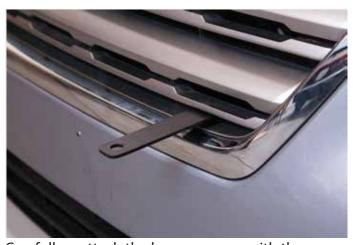
Carefully reattach the bumper cover with the Upper Brackets through the grill as shown.
