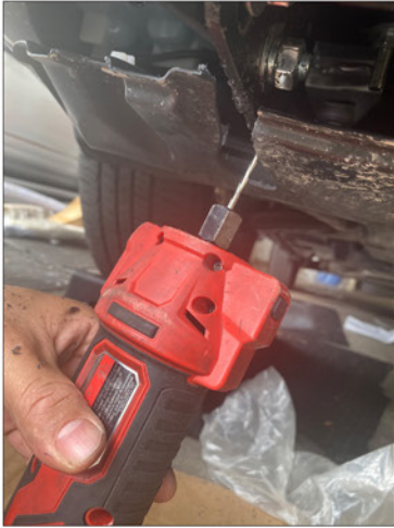
7. Cut part of the fender to make room for the bracket.
