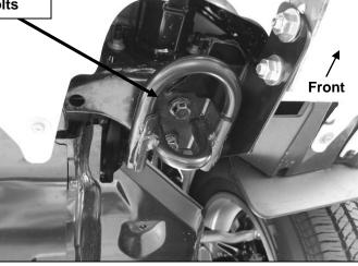
(Fig 4) Driver/left mounting Bracket installation
