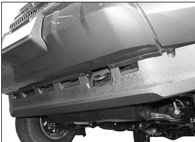
(Fig 1) Remove air dam from bottom of bumper
