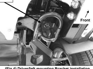
(Fig 4) Driver/left mounting Bracket installation
