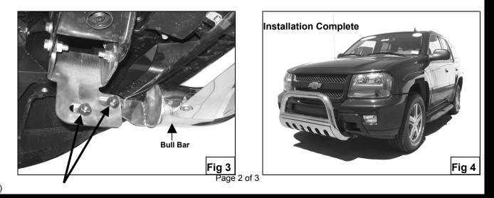
12mm x 35mm Hex Bolts 12mm Lock Washers 12mm Hex Nuts 12mm Flat Washers
