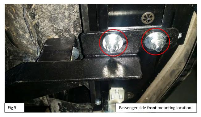
STEP6: Lastly, attach the running board with front, middle, rear mounting brackets using hardware that came with the board. And then tighten all hardware. (Fig5)
