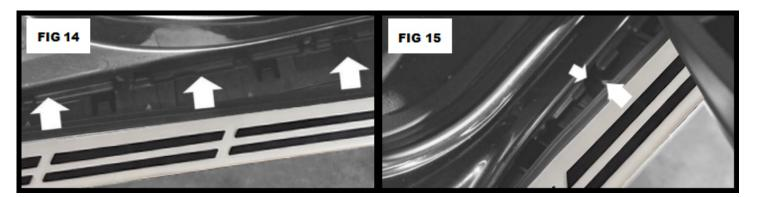
Step 14: When installing the running boards toward the front, be sure that the underside (where your screw goes) is aligned with the running board piece inside the trim piece and not over it (FIG 16).
