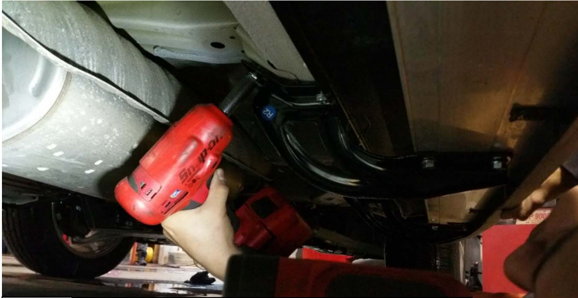
Fig 5 Passenger Side – Middle Bracket Installation Finished
