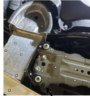
Then remove the two screws and one nut indicated by the arrow in the figure
