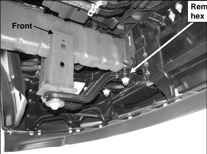
(Fig 5) Driver side mounting location pictured from behind bumper on tow hook equipped model
