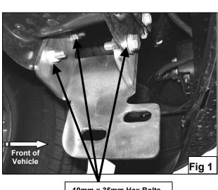
10mm x 35mm Hex Bolts 10mm Lock Washers 10mm Hex Nuts 10mm Flat Washers
