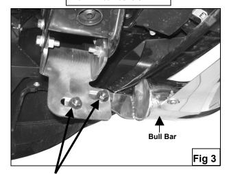
12mm x 35mm Hex Bolts 12mm Lock Washers 12mm Hex Nuts 12mm Flat Washers
