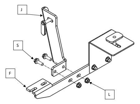
Genter the board and install nuts (L) on board (A). Fully tighten hardware
