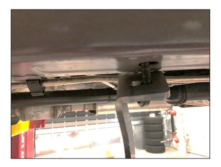
Next install the front support bracket (D) using bolt (I), washer (O), and tab nut (M) into the front hole location. To tighten pull down on the brace and tighten bolt. Do not fully tighten hardware at this time.
