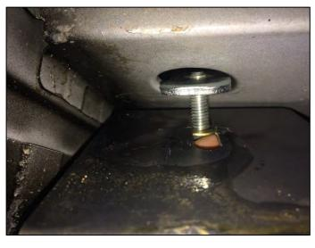
Install the bolt (I), washer (O) and tab nut (M) on driver rear bracket (J). Then install the tab nut into rear hole location. <u>Do not fully tighten hardware at this time.</u>
