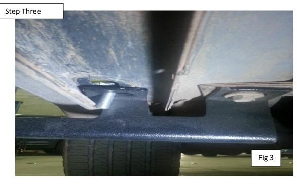
MOUNT UP REAR BRACKET USING THE DROP IN SCREW. REUSE THE FACTORY SCREW TO MOUNT THE REAR SIDE OF THE BRACKET. USE FLAT WASHER LOCK WASHER AND NUT FOR THE FRONT DROP IN. WE INCLUDE SPACERS FOR ANY ADJUSTMENTS.
