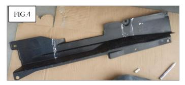
(1) As FIG.4 shows, remove the preventer plate under the vehicle.
