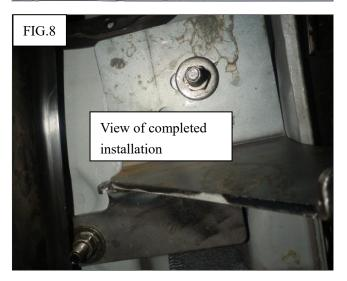
STEP 4. Connect the running board onto the brackets and adjust it to a proper location. Notice that the running board should be parallel to the body of vehicle. Tighten the bolt while adjust them to the best location.
