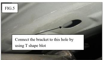
(2) Connect the bracket vehicle by using M6 tapped hole under the chassis,
