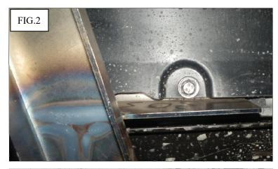
(2) Turn over the preventer plate and connect the brackets inward the skid plate, do not tighten the bolts.
