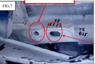
Connect the rear bracket under the chassis by using the hole showed on FIG.7 with (8) special bolt.
