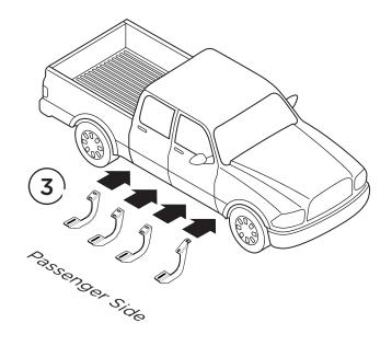
**4.** Install the first passenger side front Bracket closest to the front wheel. Align with existing factory holes in the rocker panel as shown (4a), Secure the first Bracket using one (2) M8 x 30mm Hex Bolt, one (2) M8 Lock Washer and one (2) M8 Flat Washer (4b).
