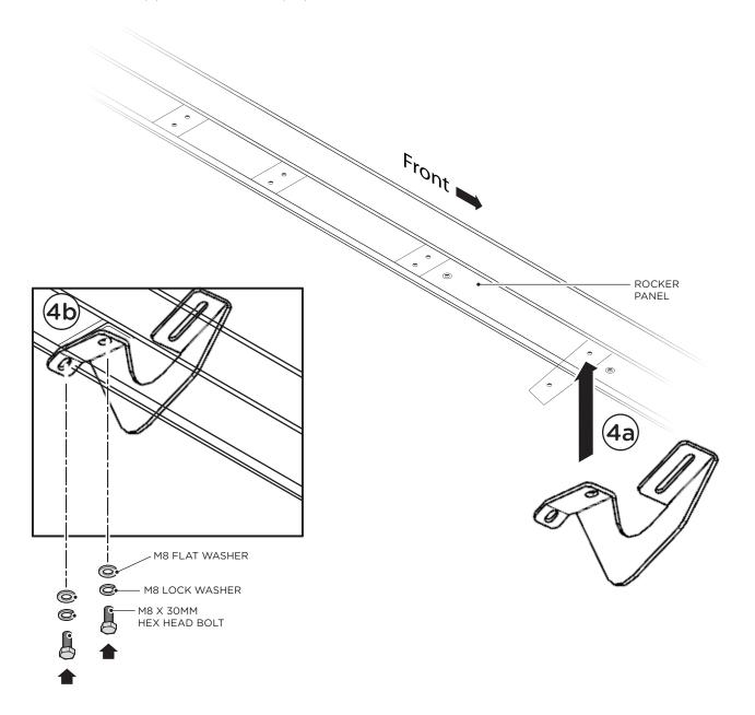
**5.** Position the remaining two (2) passenger side center ro rear Brackets as shown (5a) and secure using two (2) M8 x 30mm Hex Bolts, two (2) M8 Lock Washers and two (2) M8 Flat Washers per Bracket (5b).
