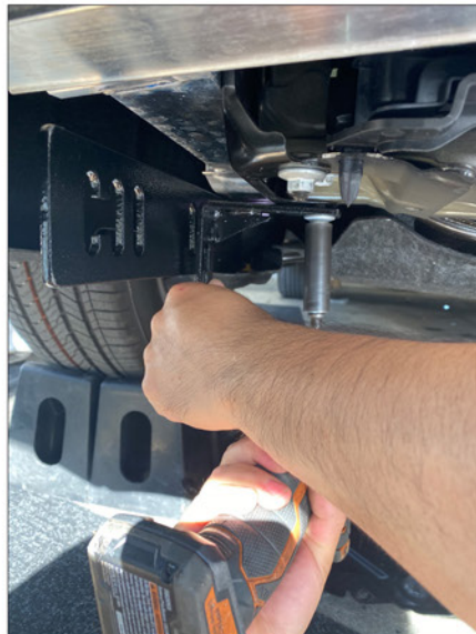
4.Secure with an air gun.
