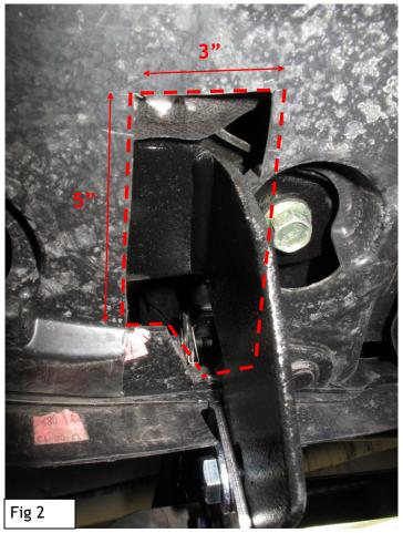
STEP4: Cutting on the plastic area shown in Fig3 for approximately 1" wide and 2" long.
