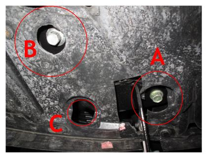
STEP6: Apply WD-40 on the factory screws. And firstly put back the screw on the left [Marked: B], secondly put back the screw on the right [Marked: A]. Lastly, put back the factory screw removed from step2 [Marked: C]. (Fig4)
