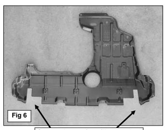
Cut out the sections illustrated to clear the Mounting Brackets (Pictured for example only, actual area to cut may be different)
