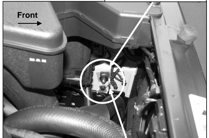
(Fig 5B) Driver Support Bracket pictured from above
