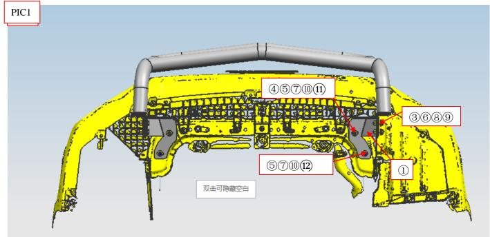
Step 3:Install the bar body on the bracket and adjust the mounting position of the bracket according to the position of the bar
