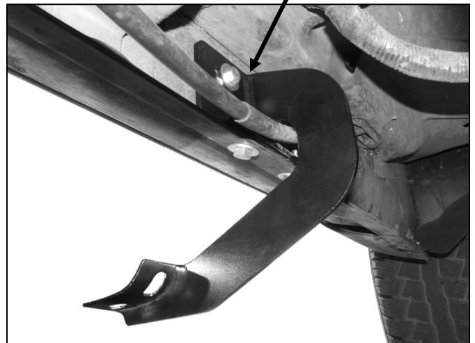
(Fig 2) Driver side-front Mounting Bracket location
