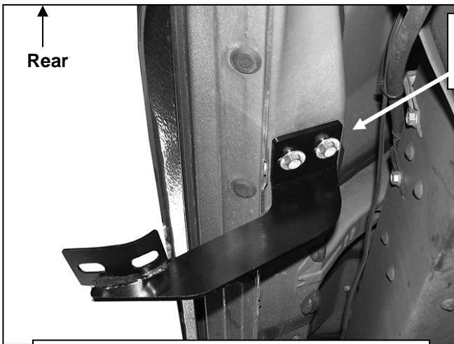
(Fig 5) Driver/Left Rear Bracket installed
