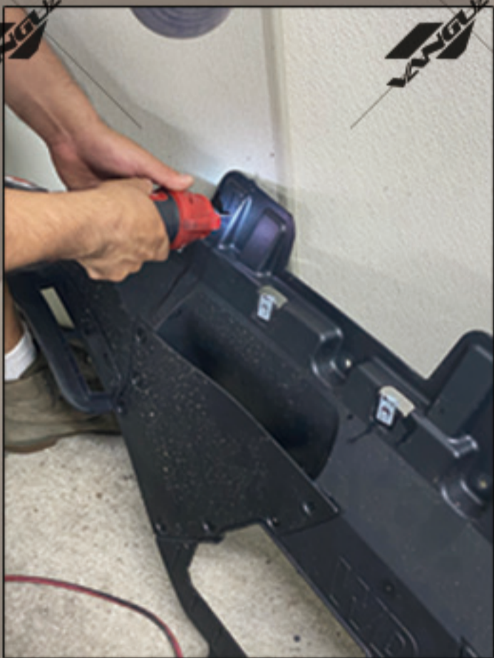
3. Cut off part of the fender space to leave a place for the bracket to install.
