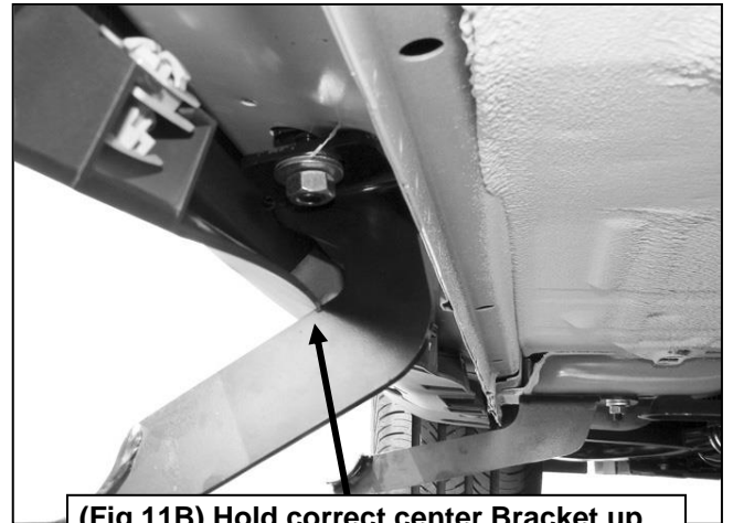
(Fig 11B) Hold correct center Bracket up in place to determine area to cut from bottom edge of rocker panel cover
