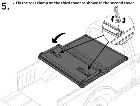
• Adjust the connection position of the rear clamp and T-bar according to the 6. actual situation, open the cover and place it on the lathe, and push the rear clamp vertically to fix it to the rails on both sides of the lathe.
