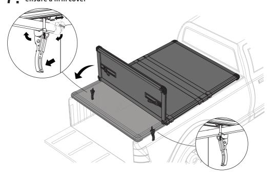
8. FINISH THE INSTALLATION . After rear clamps have been latched securely, close/lock tailgate and cover cannot be opened from the outside
