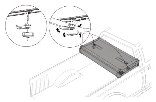
• Connect the provided Rear clamps to the T-bar on the cover as shown in the figure
