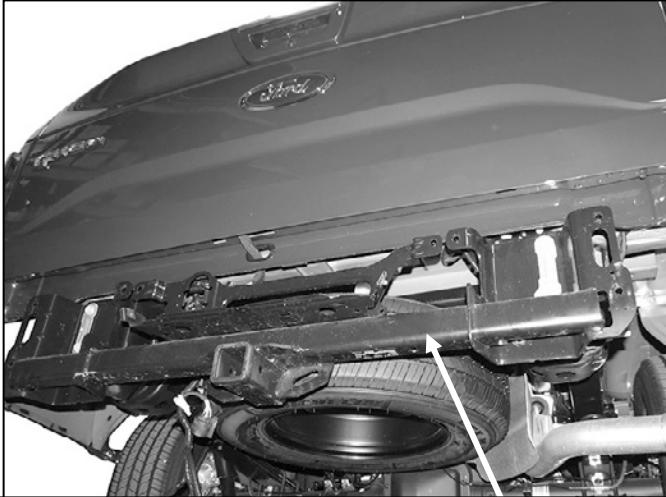
(Fig 15) Reinstall integrated receiver hitch/bracket assembly on models with "HD Towing" package
