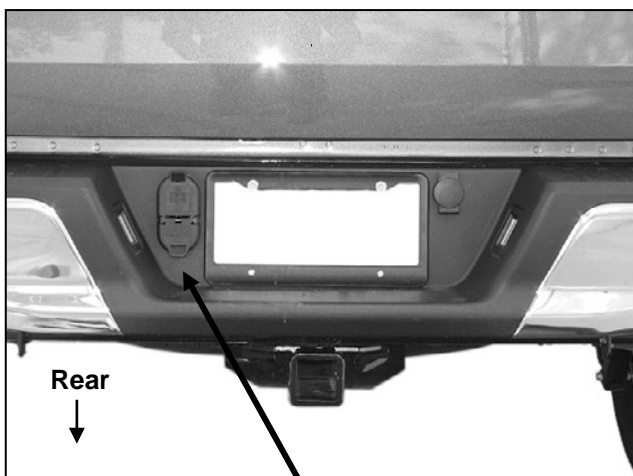
(Fig 1) Unplug and remove 7-wire trailer plug
