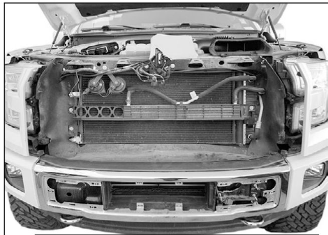
(Fig 5) Unplug harness leading to shutter assembly in grille. Remove grille assembly
