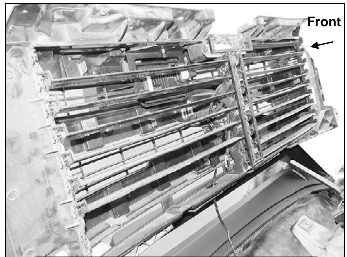
(Fig 19) Plug harness into sensor. Check fit of harness, secure harness to grille. Rewrap wiring harness. Reinstall shutter blades. Reinstall grille assembly
