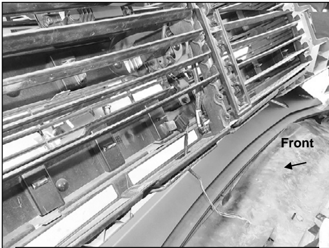
(Fig 18) Push sensor plug up through opening. Pull harness up between shutter blades and grille to sensor. NOTE: Temporarily remove shutter blades as necessary for access to harness and sensor
