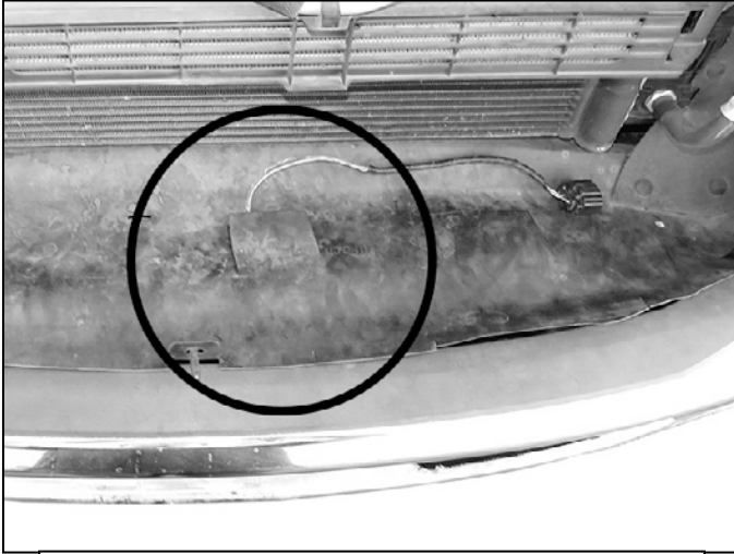
(Fig 16) On installations using factory bumper, cut an opening in the rubber splash guard approximately 3" back from front edge
