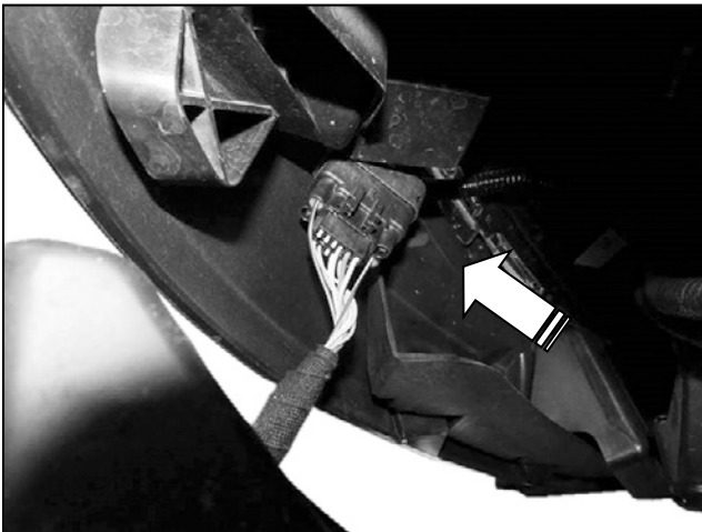
(Fig 7) Pull the bumper out slightly and unplug the outer wire harness
