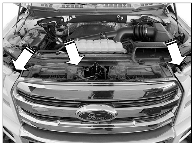
(Fig 2) Remove cover from top of grille (arrow). Remove hardware attaching top of grille to radiator core support. Release clips attaching top of plastic headlight surrounds (arrows above headlights)
