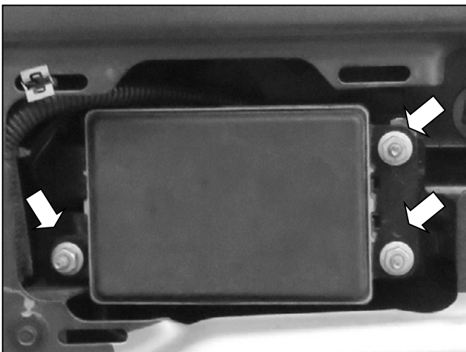
(Fig 3) Remove and unplug adaptive cruise control from driver/left side of frame, if equipped
